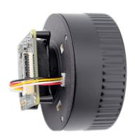
The solution allows you to mount Canon EF or EF-S lens onto the OneInchEye Camera and have features like autofocus and aperture control available in rpicam-apps, libcamera or V4L2 (Video4Linux2) API.
