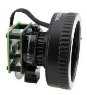
The solution allows you to mount Canon EF or EF-S lens onto the Raspberry Pi High Quality Camera and have features like autofocus and aperture control available in rpicamapps, libcamera or V4L2 (Video4Linux2) API.
